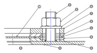
Installation with welded threaded bolts.
